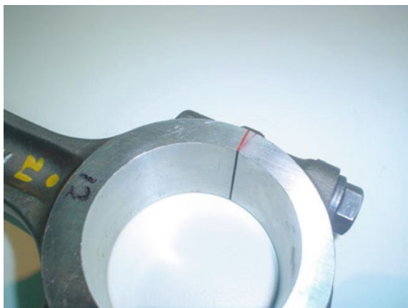
Fig. 13.5 Additional notches on the big end, on the top and bottom surface
