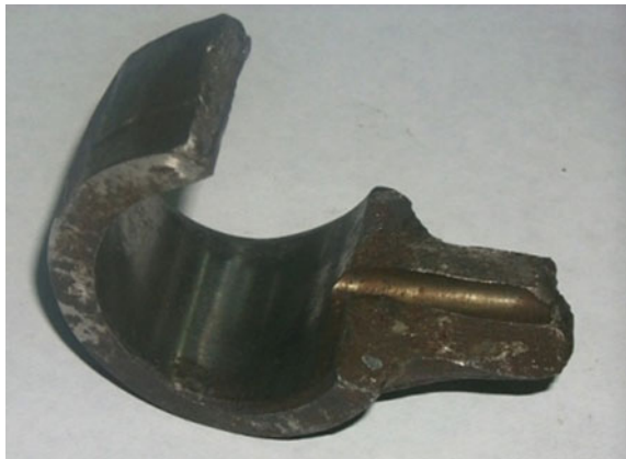
Fig. 13.6 A failure of a connecting rod at junction of small end
