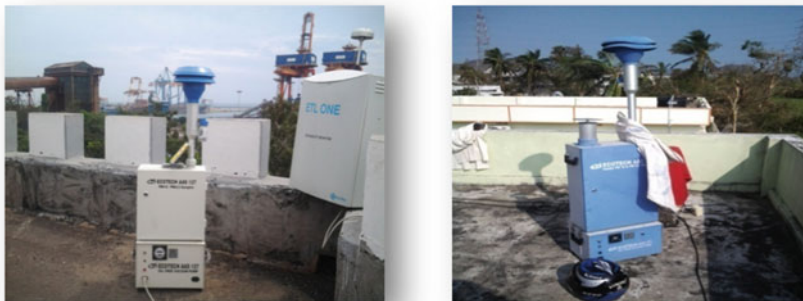
Fig. 3 Instruments of fine particulate samplers at monitoring stations
