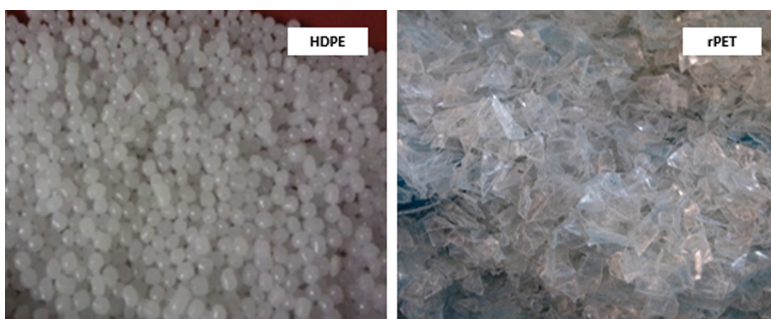
Fig. 1. Raw materials: HDPE pellet and rPET flakes
