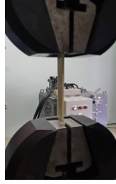
Fig. 3. Tensile test of composite material using universal testing machine
