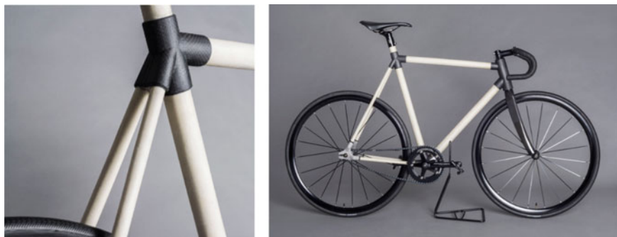
Fig. 11.4 The product of bonded joints containing CNF in the assembled bicycle from Finland Ideas2cycles company. Reproduced from [45]
