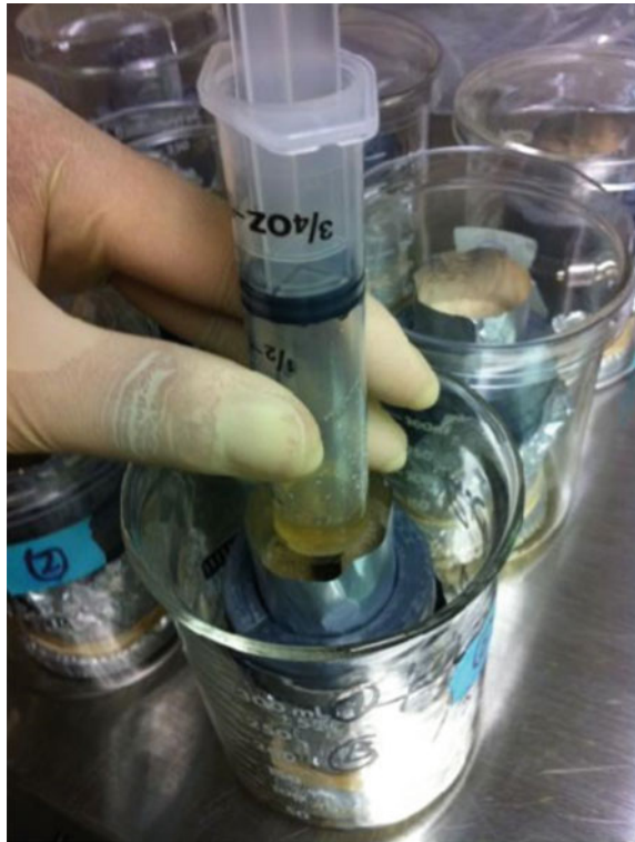
Fig. 2 Injection of culture medium into Fly ash specimen
