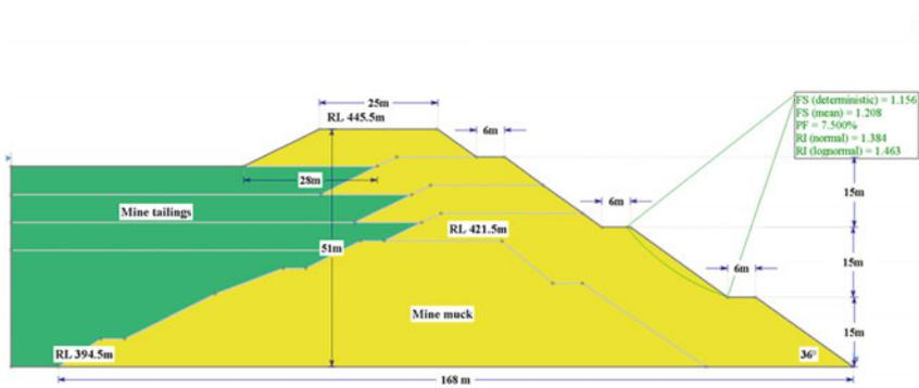
Fig. 4 Probabilistic analysis result of downstream slope
