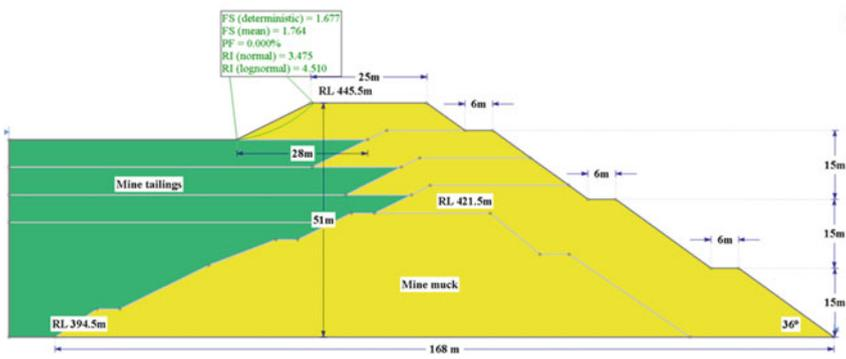
Fig. 3 Probabilistic analysis results of upstream slope
