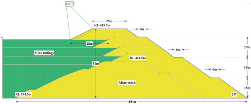
Fig. 1 Deterministic analysis results of upstream slope
