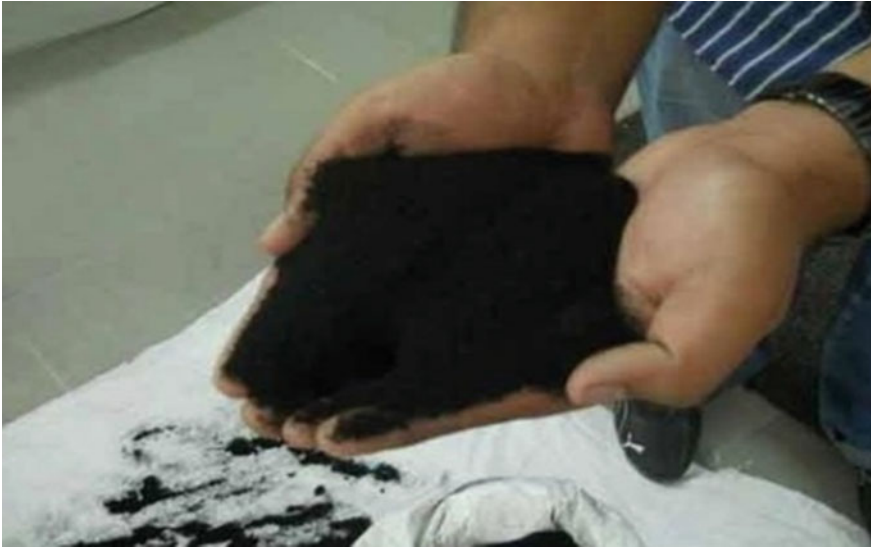
Image 2 Fine rubber powder used as additive ( Source as provided by powder supplier)
