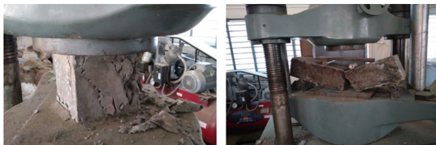
Fig. 3 Failure of specimen in compression and flexure under load applied using universal testing machine
