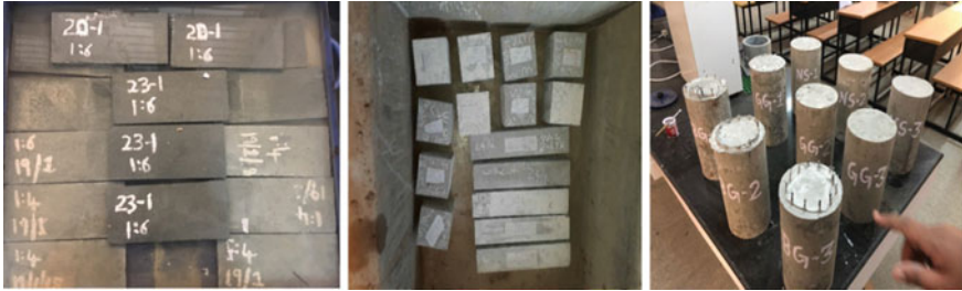
Fig. 2 Reinforced concrete test specimens
