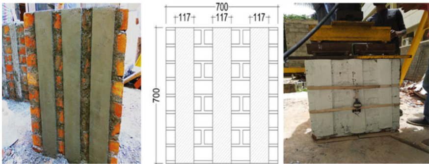
Fig. 7 Polyester reinforced masonry wallets
