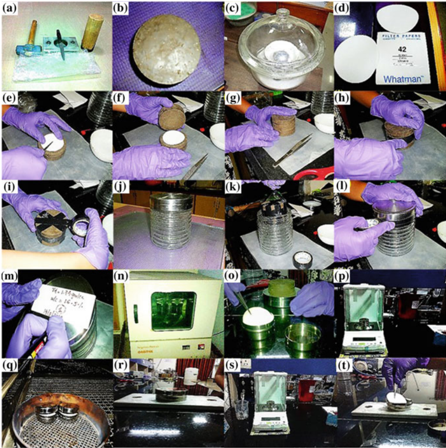
Fig. 1 Step-wise sequential procedure of In-contact filter paper method for matric suction determination
