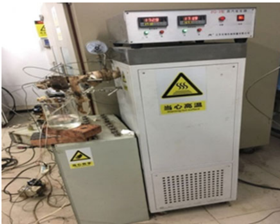
Fig. 3 Schematic diagram of the steam generator
