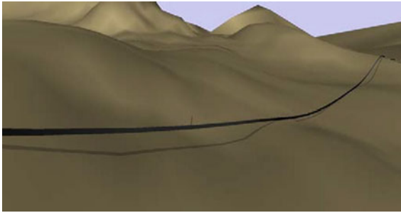
Fig. 1 Free spanning pipeline on an uneven seabed [2]
