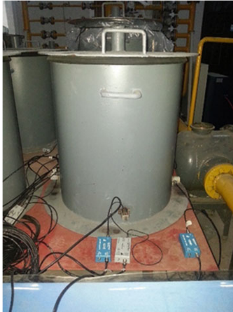
Fig. 1 Experiment on secondary amplification of corrosion of simulative tank floor
