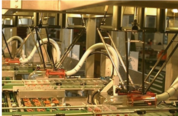
Fig. 10.11 Delta Robot on an assembly line ( http://www.parallemic.org/Reviews/Review002.html )
