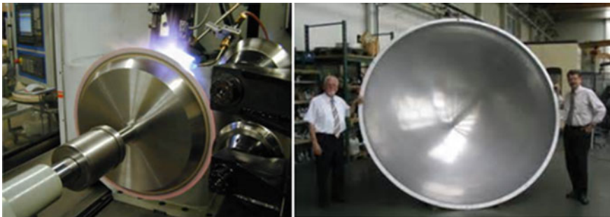
Fig. 14.9 Spinning process and products ( https://www.thomasnet.com )
