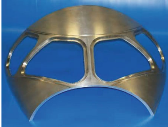
Fig. 14.11 Prototype part of an Airbus fuselage, created by explosive forming ( www.sciencecodex.com )
