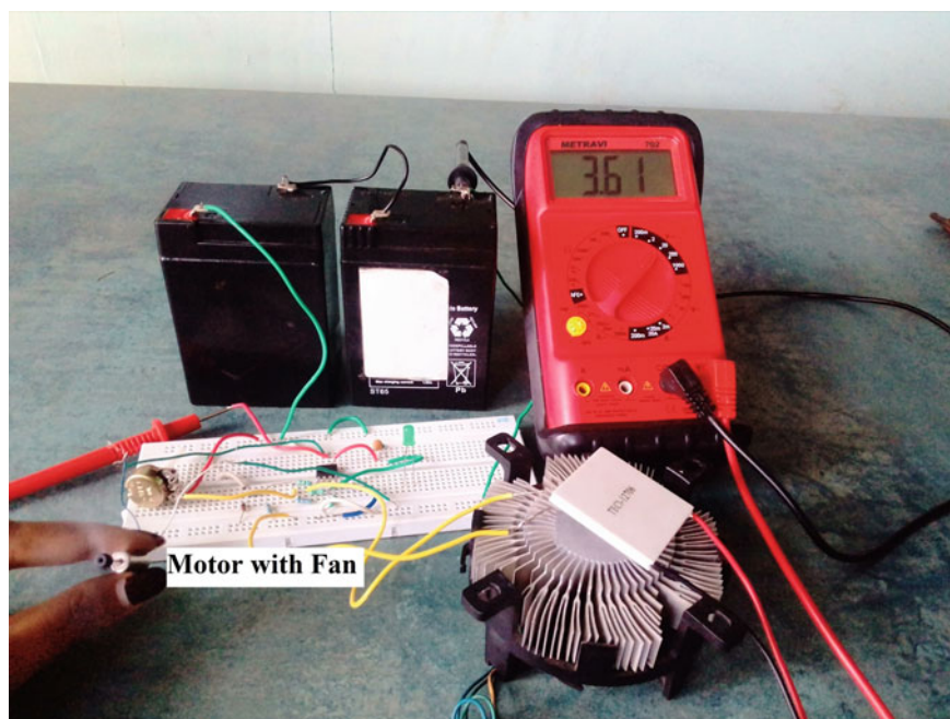
Fig. 9 The running motor with fan utilizing regulated output voltage
