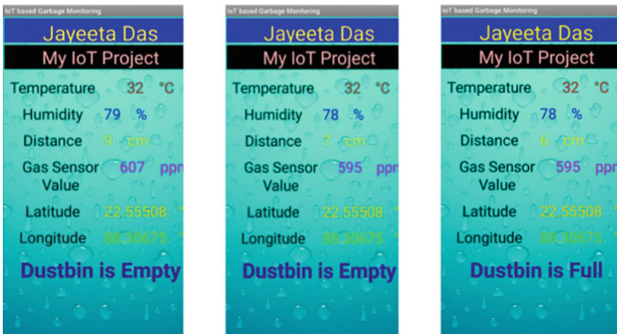
Fig. 8 Main screen display of mobile app when the garbage bin is at normal temperature
