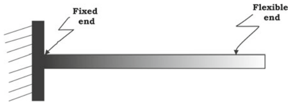
Fig. 5 A cantilever beam
