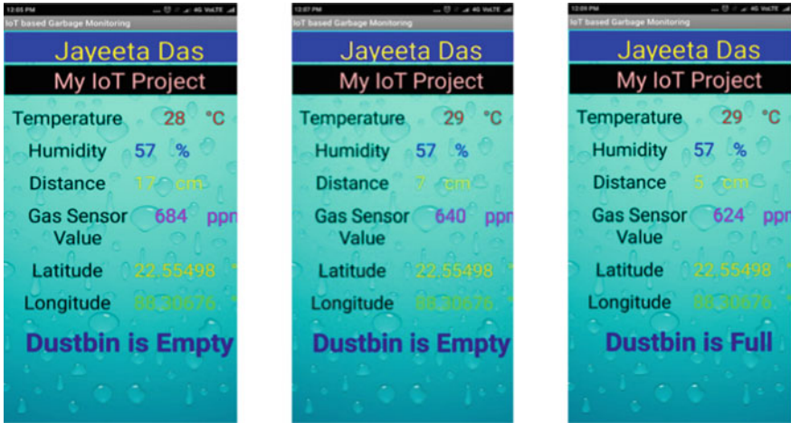
Fig. 7 Main screen display of mobile app when the garbage bin is in ac room
