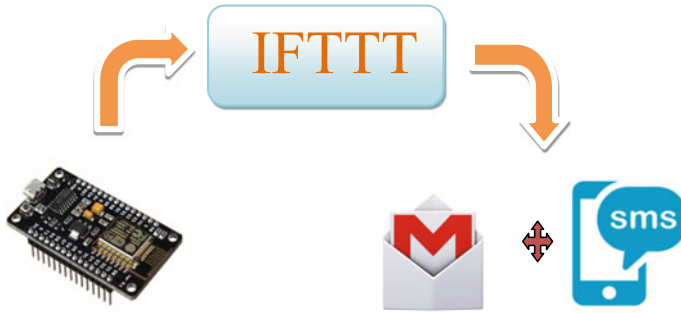
Fig. 2 IFTTT with NodeMCU Gmail and SMS notification
