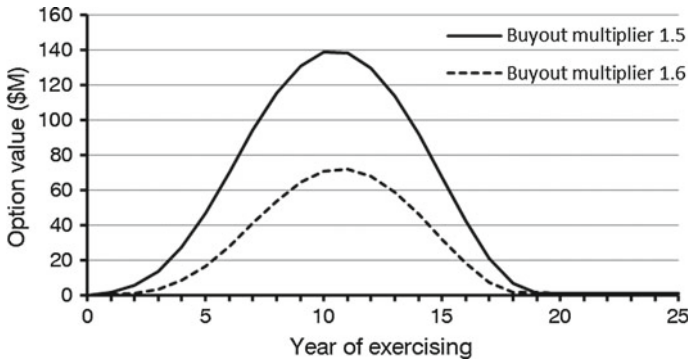
Fig. 6.3 Buyout example (constant buyout cost); option value versus time for different levels of buyout
