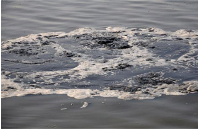
Fig. 3 Sludge upwelling in anaerobic reactor increases mixing with fresh input water, increases active bacterial number over a hundred-fold and reduces holding time to 8–16 h
