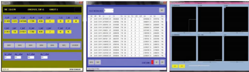
Fig. 3 Different parameters value window, notepad file window, and graph window as displayed by data logger for healthy and non-healthy solar panel, respectively
