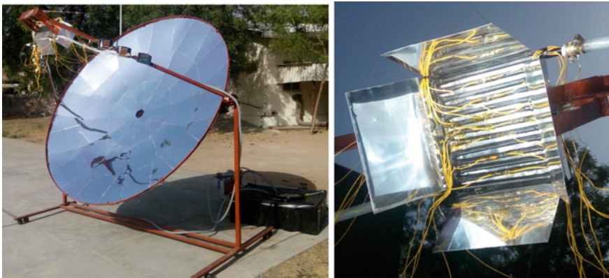
Fig. 5.9 Parabolic dish and receiver with zoomed in view of receiver
