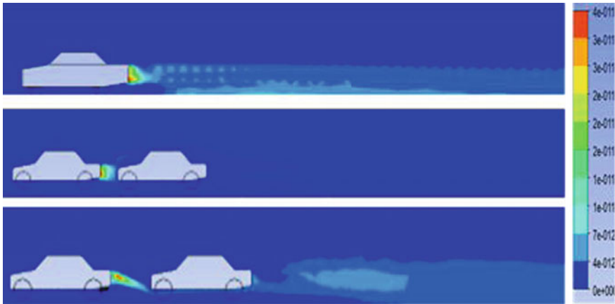
Fig. 7 PM2.5 concentration cloud diagram of y = 0.8125 m section (bicycle, 0.8, 1.6 m)
