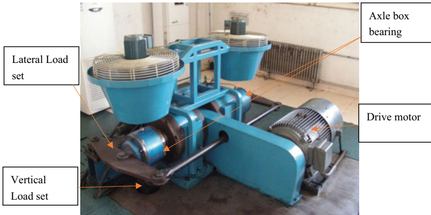
Fig. 8 Test rig of railway axle rolling bearings
