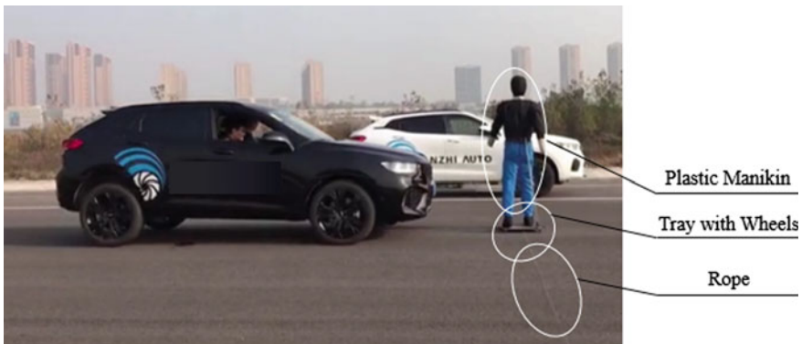
Fig. 1 Current closed field test method for CAV
