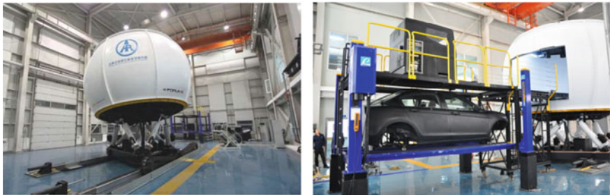
Fig. 3 The RIOH researching simulator with 8-DOFs
