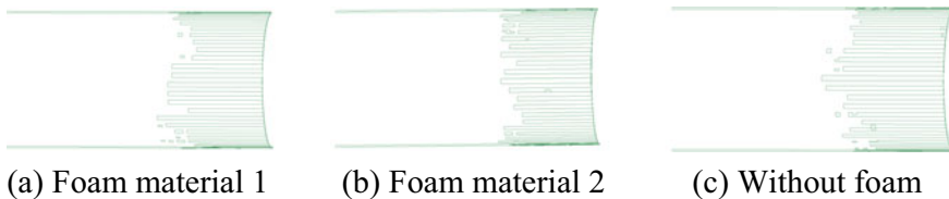
Fig. 3 Failure in the lining with and without embedded foam due to 25 kg TNT
