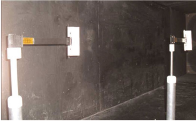
Fig. 10.2 Tandem harvesters comprising of flexible beams with a tip flap tested in Bryant et al. (2012). Reproduced with permission from Bryant et al. (2012)
