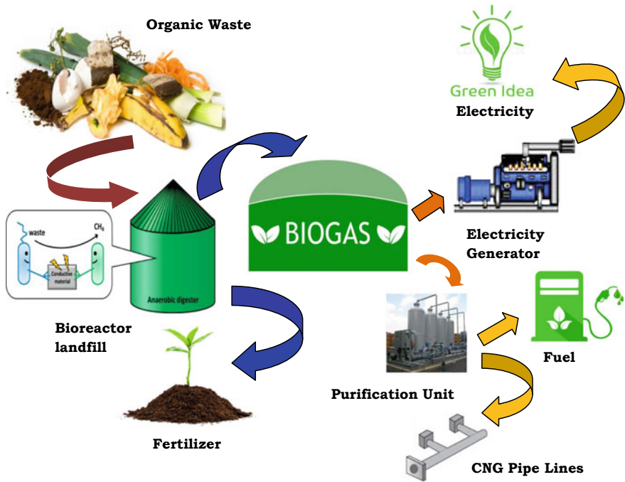
Fig. 1 Flow diagram of waste to biogas production and utilization (Sahota et al. 2018)
