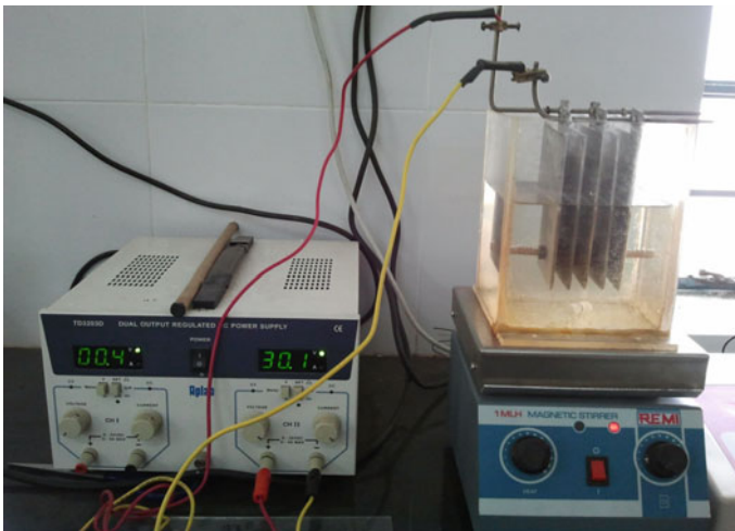
Fig. 4 Experimental setup used for leachate treatment in ECT
