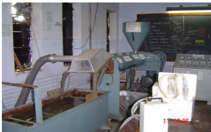
Fig. 6 Green recycling of plastics set-up as developed by Ghosh (2004)
