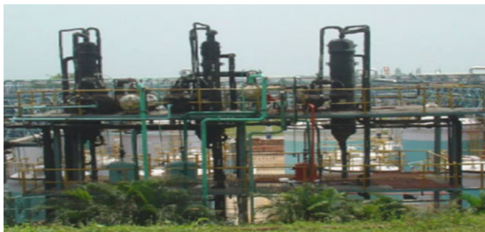
Fig. 6 Falling film evaporator
