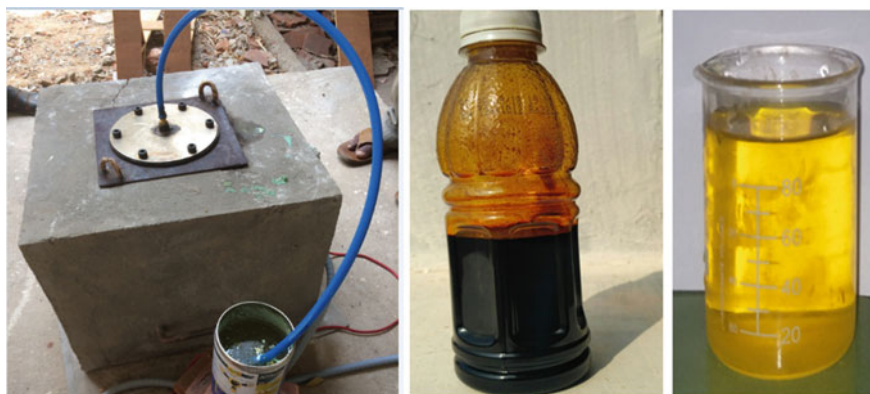
Fig. 1 Plastic pyrolysis reactor, pyrolysed oil, distilled pyrolysed oil
