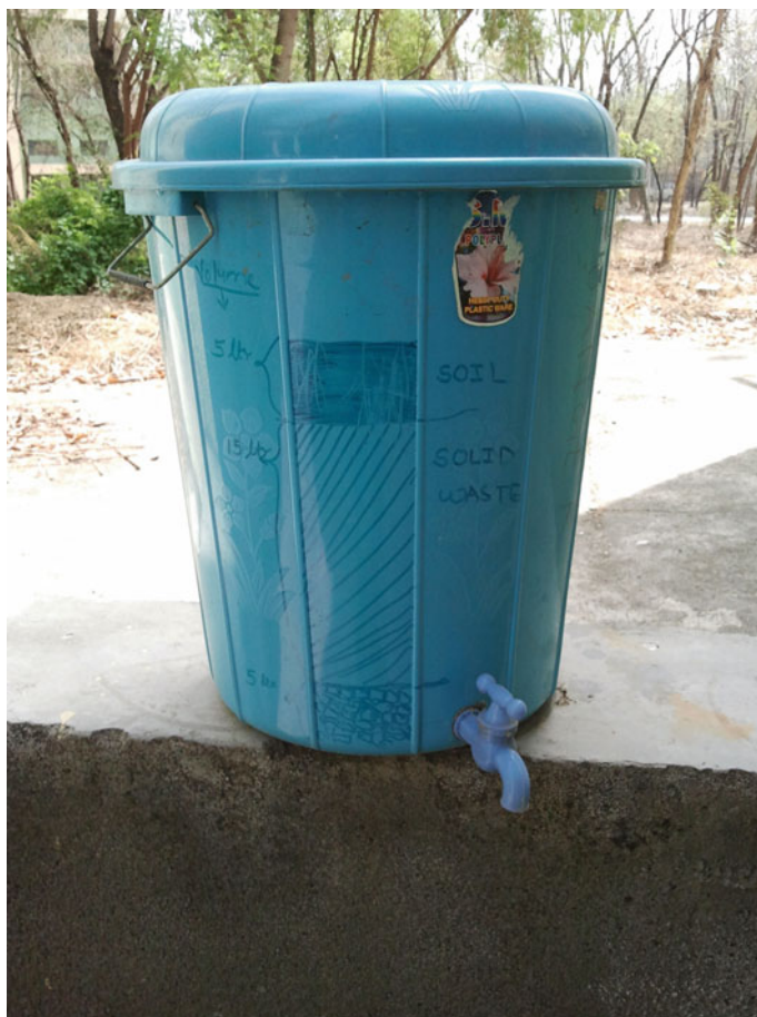
Fig. 2 Leachate-generating bucket filled with solid waste collected from VNIT dumping site
