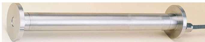
Fig. 5 Intelligent SMTI with mechanical memorization of the maximum and minimum values of the controlled SSS parameter
