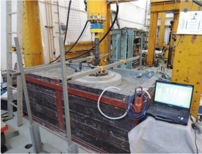
Fig. 6 Experimental box assembled with the actuator
