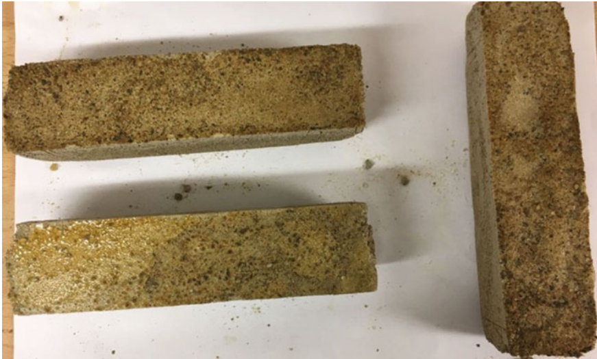
Fig. 1 Beams 4 × 4 × 16 of ordinary middle-sized sand in 28 days
