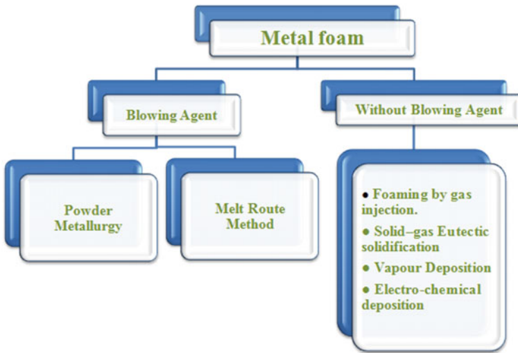
Fig. 4.1 Processing method of metal foam based on gas source used
