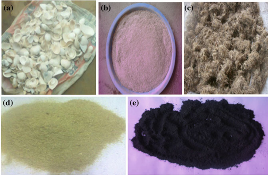
Fig. 17.1 The images of raw seashell (a), Periwinkle shell (b), Palm kernel fiber (c), banana peel un-carbonized (d), and Banana peel carbonized (e)
