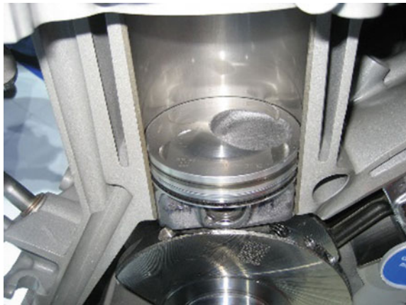
Fig. 6.2 Piston showing swirl cavity ( https://en.wikipedia.org/wiki/Gasoline_direct_injection )
