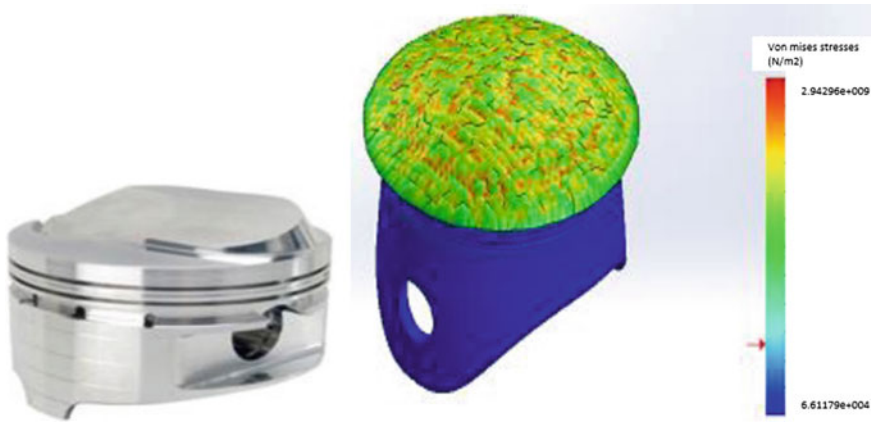
Fig. 11.2 Induced stresses in typical piston (Hemasundaram and Suresh 2015)
