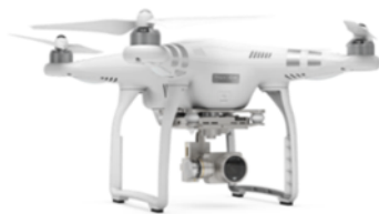
Fig. 3 UAV used in this study (DJI Phantom 3 Professional quadcopter)
