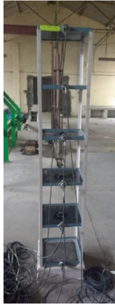
Fig. 1 Instrumented steel structure laboratory model
