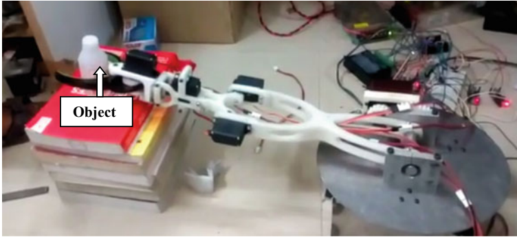
Fig. 13 Photographic view of in-plane grasping by MGRS
