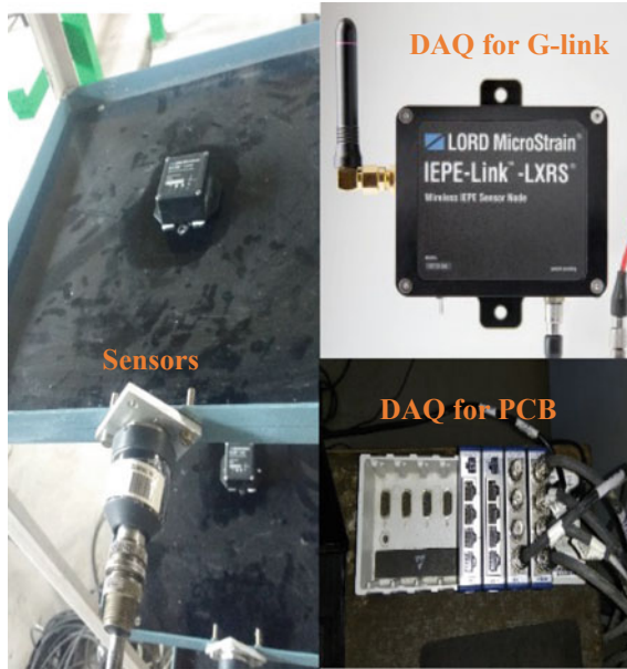
Fig. 2 Sensors and data acquisition system
