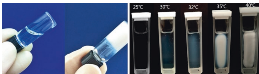
Fig. 2.3 Showing gel formation of thermosensitive polymer upon heating
