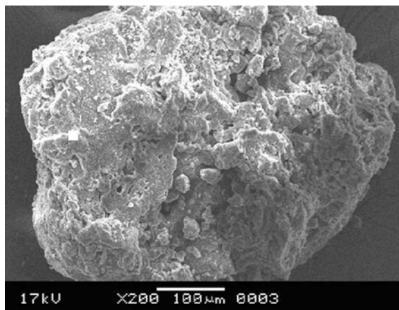
Fig. 9.1 SEM photograph of aceclofenac-loaded chitosan-TSP IPN microparticles. (Reprinted from Jana et al. (2014). Copyright (2014), with permission from Elsevier)
