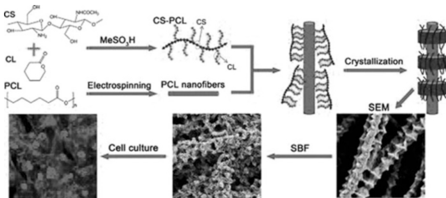
Fig. 10.5 Schematic of shish kebab-structured scaffold preparation using chitosan–polycaprolactone copolymers. (Reprinted with permission from Jing et al. 2015; Copyright © 2015 American Chemical Society)
