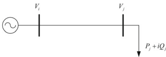
Fig. 1 Systematic two-bus system
