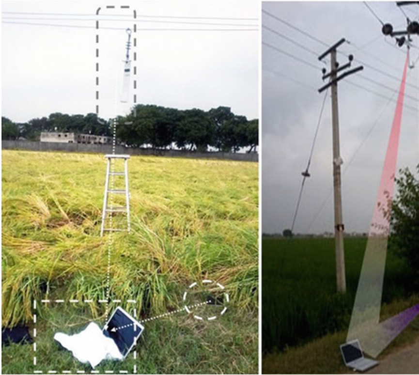
Fig. 3 Field test conducted using designed conductor altitude measurement system
