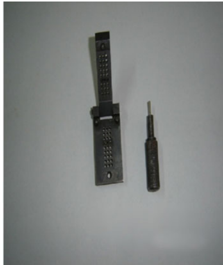
(b) Hand tool for modifying paper-tape program
