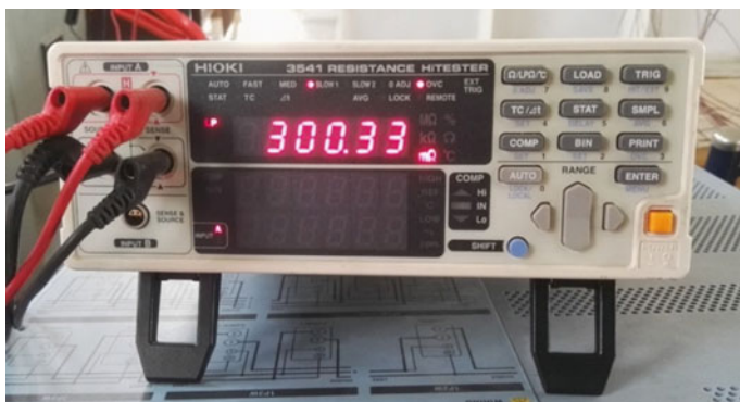
Fig. 14.2 DC resistance tester (HIOKI 3541, Japan)
