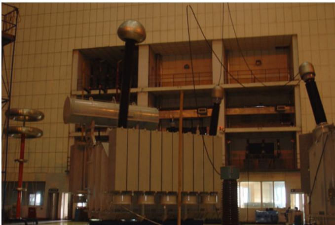
Fig. 15.78 Product outline for a 500 kV autotransformer
