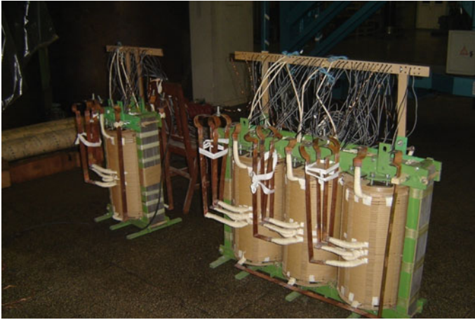
Fig. 15.6 Transformer model for DC bias test
