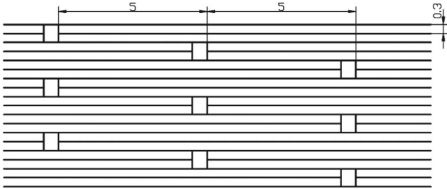
Fig. 9.3 Three-step lap joint (two sheets as one stack in core stacking, unit: mm)
