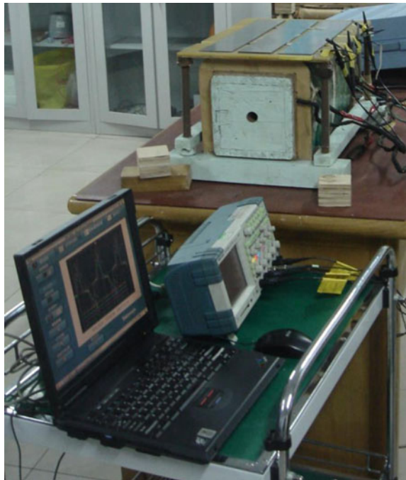
Fig. 13.33 Measurement and prediction of magnetic behaviors in laminated sheets
