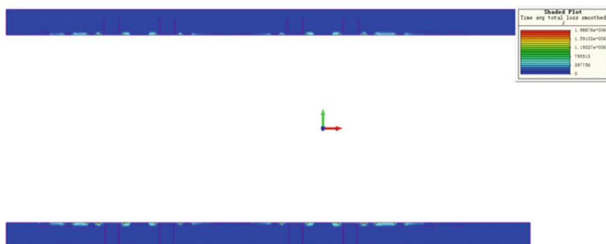
Fig. 14.29 Loss density distribution in the core clamping at high-voltage side (700MVA/750 kV, D02)
