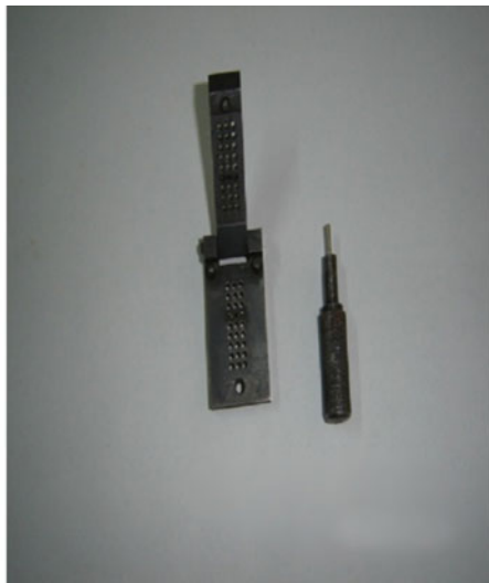
(b) Hand tool for modifying paper-tape program
