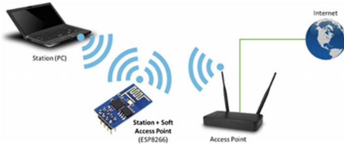
Fig. 6 ESP8266 operating in the station + soft access point mode
