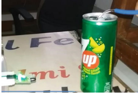
Fig. 6 IR sensor sensing the bottle and filling
