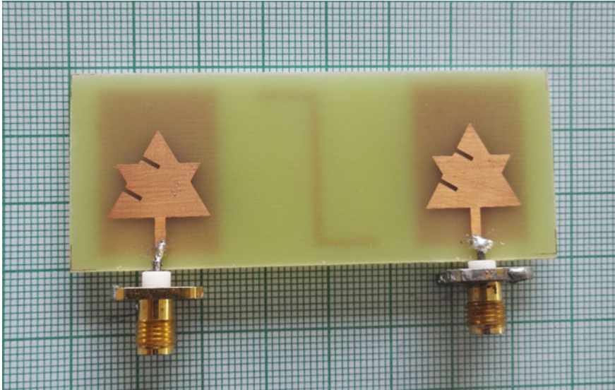
Fig. 6 Photograph of the fabricated WLAN MIMO antenna—front view
