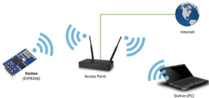
Fig. 5 ESP8266 operating in the station mode
