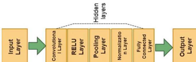
Fig. 2 Architecture of convolution neural networks (CNNs)
