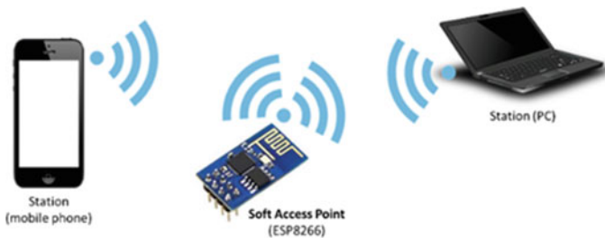
Fig. 4 ESP8266 operating in the soft access point mode
