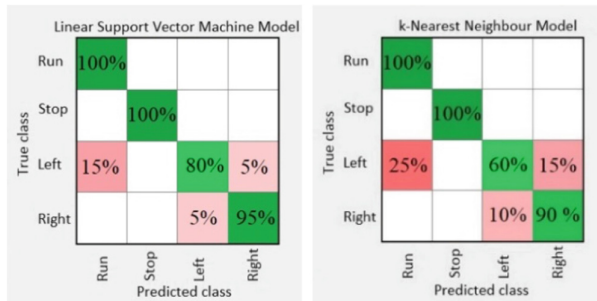
Fig. 6. Confusion matrix for subject II in real time analysis with linear SVM and kNN.
