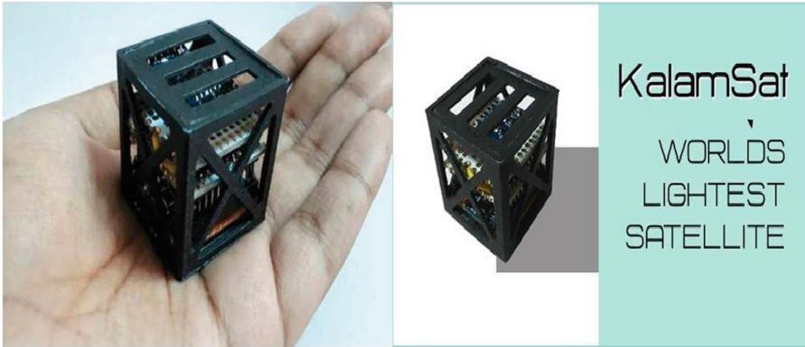
Fig. 2. Indian FemtoSat “KalamSat” (4 cm × 4 cm × 4 cm; 64 grams) [7].
