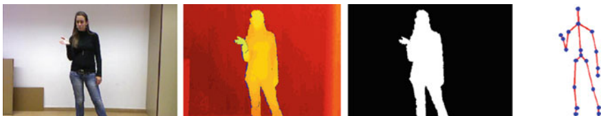
Fig. 5.5 Different data modalities provided for gesture recognition. Image adopted from Escalera et al. [32]
