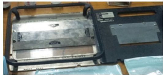
Fig. 5.6 Wedges used for telecobalt and LINACS
