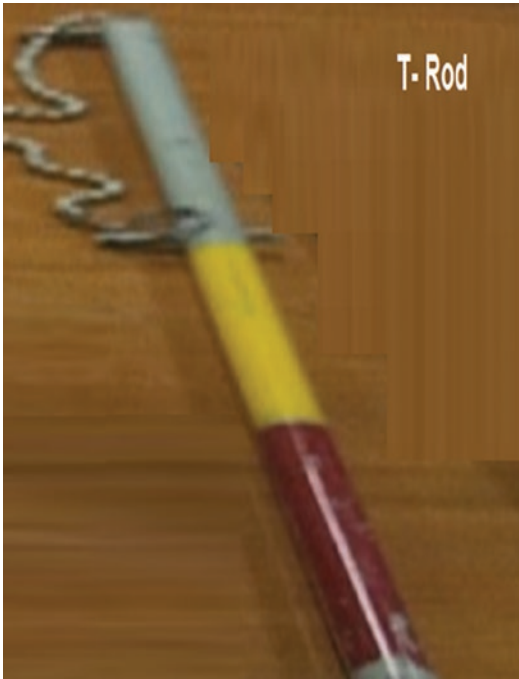
Fig. 7.3 T-rod with colors indicating source position
