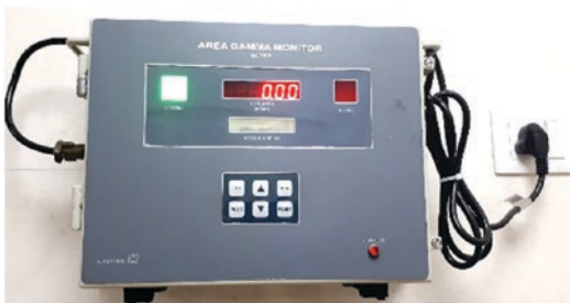
Fig. 4.2 Area gamma monitor installed for brachytherapy installation
