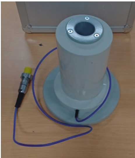
Fig. 3.8 Showing the schematic diagram of well type chamber
