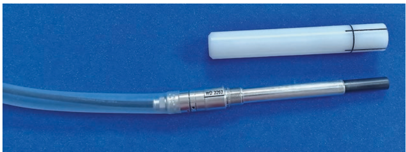
Fig. 3.4 Showing the schematic diagram of Farmer chamber
