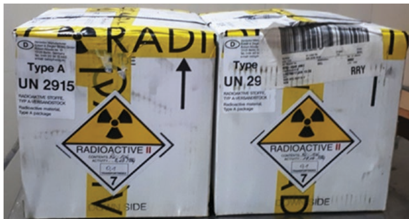
Fig. 4.1 The packaging of radioactive material for transport, the type "A" package
