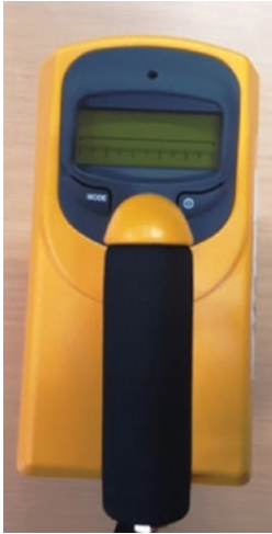
Fig. 4.4 Pressurized ion chamber based survey meter
