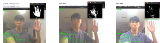
Fig. 7. Effects of lighting to the preprocessing stage.
