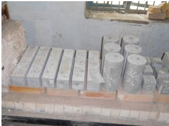
Fig. 2 Specimens arranged for heating in furnace
