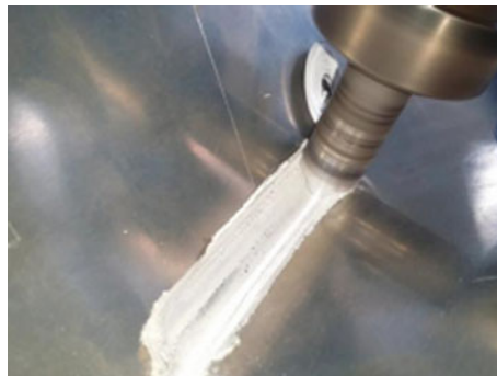
Fig. 4 Weld setup during friction stir welding process
