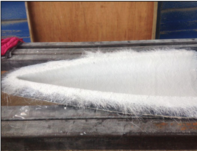
Fig. 4 Lamination process using fibre and resin
