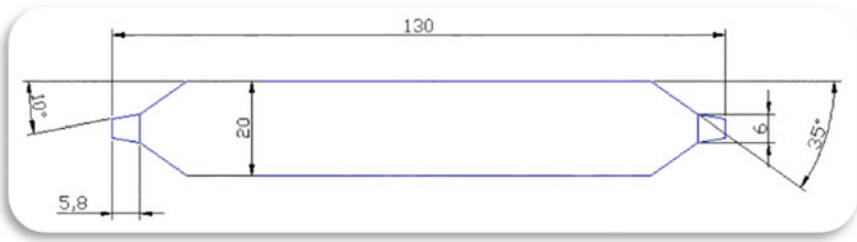
Fig. 3 Surface-hardened H13 welding tool
