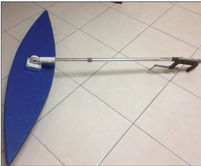
Fig. 6 The final prototype of outrigger stabilizer with an adjustable arm
