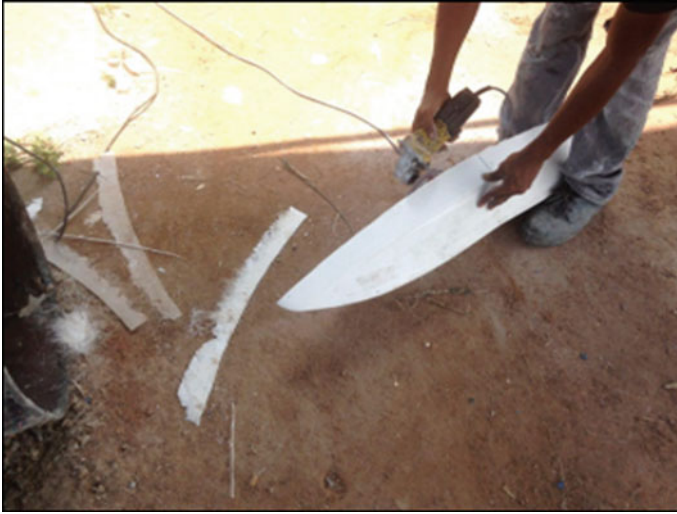
Fig. 5 Sanding the hull form
