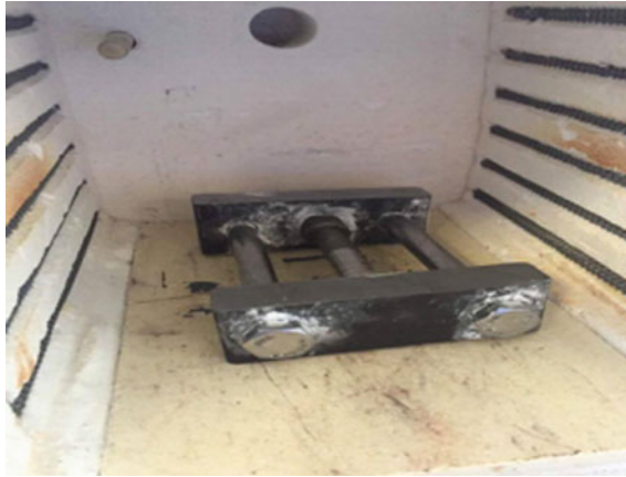
Fig. 5 Clamped specimen in the furnace
