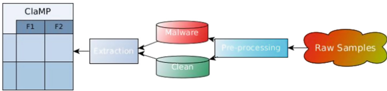
Fig. 3. CLaMP (Classification of Malware with PE headers)
