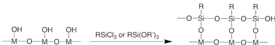
Fig. 10.11 Silylation reaction of a layered material
