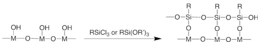
Fig. 10.11 Silylation reaction of a layered material
