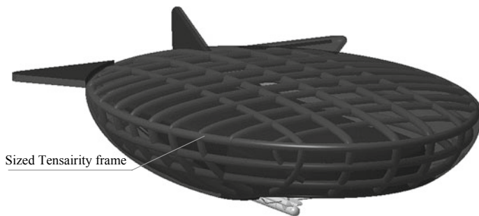
Fig. 10 The considered Tensairity frame is elliptical and must withstand the effect of frontal drag, which is a distributed load. This is similar to the test case studied in the previous section
