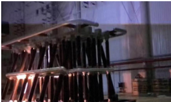
Fig. 5 Insulation test of base of Ch2 stack
