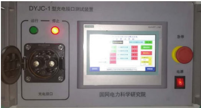
Fig. 3 Electric vehicle control pilot simulation device
