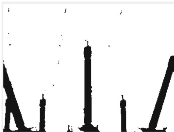
Fig. 3 The noise of bushing infrared image is removed after the opening operation
