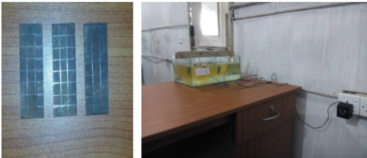
Fig. 2. (a) 50 \times 20 \times 3 mm steel specimens. (b) Arrangement of apparatus
