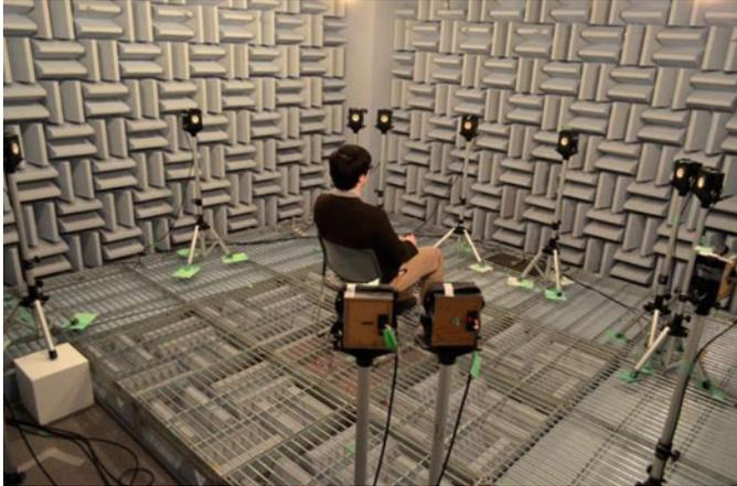
**Fig. 13.7** Reproduction of four types of original sound field in anechoic chamber
