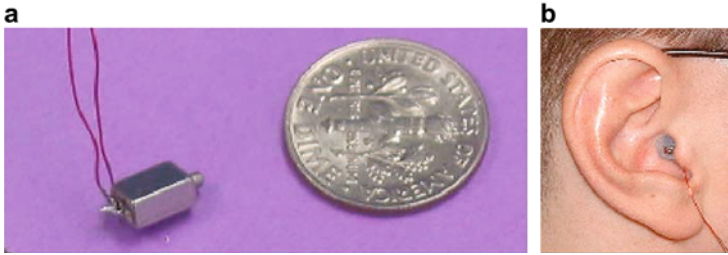
Fig. 9.9 Photographs of (a) small loudspeaker and (b) its placement in ear canal of subject. (Zotkin et al. 2006)
