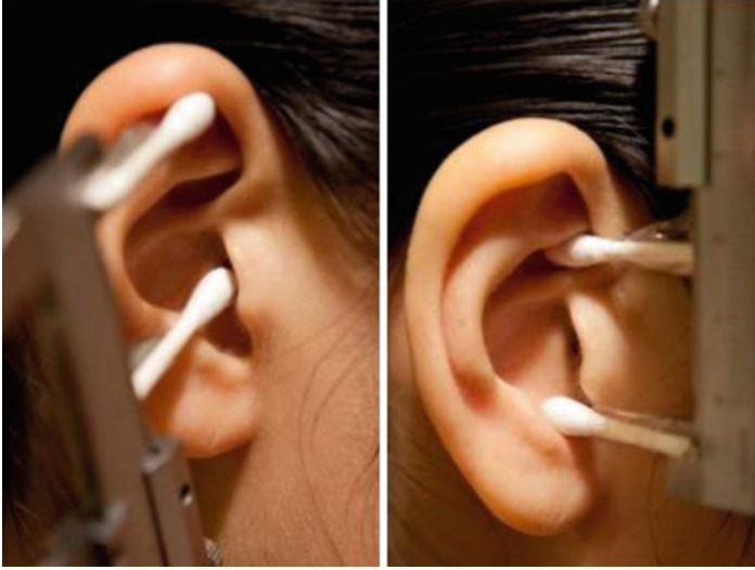
Fig. 4.28 Practical measurements for F_{P2} and F_{P3} estimation. Left panel: measurement of the distance d_{1-17} between the ear-canal entrance and the helix rim. Right panel: measurement of the vertical distance d_{4-12(\text{vert})} between the concha floor and the cymba anterior wall. (Mokhtari et al. 2016)
