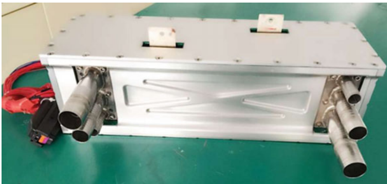
Fig. 3 Fuel cell stack for durability cycle test
