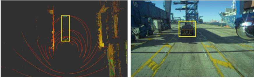
Fig. 4 These are point cloud in bird's eye view and image data collected at the same time. The unloaded semitrailer trunk in image is obvious to be detected. However, the point cloud of the trailer part is extremely sparse, which brings difficulty to the lidar-based detector for a robust detection
