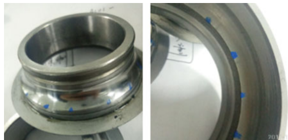
Fig. 12 Disassembly of the hub bearing
