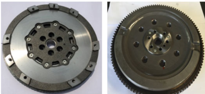
Fig. 4 Dual-mass flywheel object
