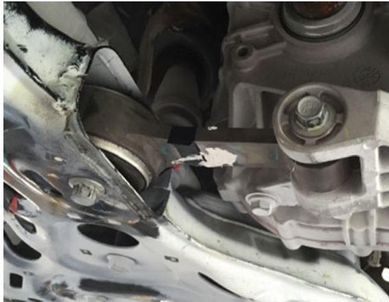
Fig. 13 Drive durability road load spectrum collected and strain gauge layout location
