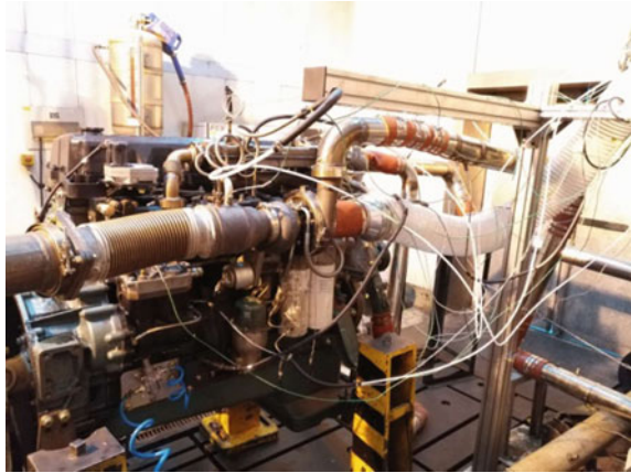
Fig. 1 Test diesel engine of symmetric exhaust
