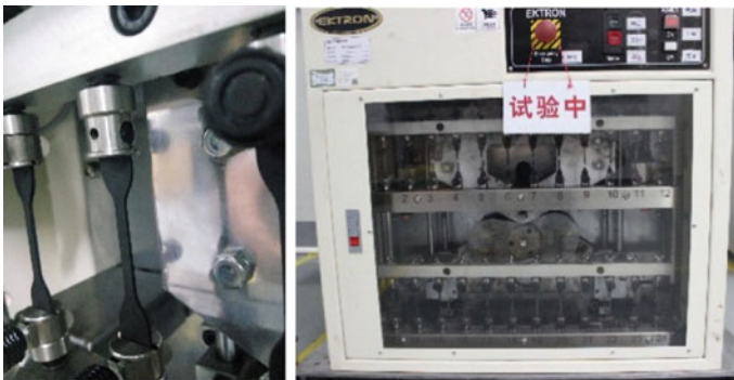
Fig. 2 Fatigue test diagram of rubber material
