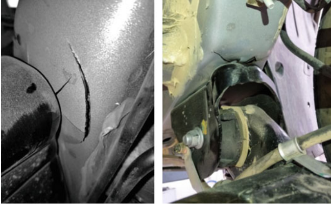
Fig. 1 Cracking of torsion beam mounting point
