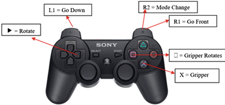
Fig. 1. The assigned movement of the mini robot in the PS2 controller
