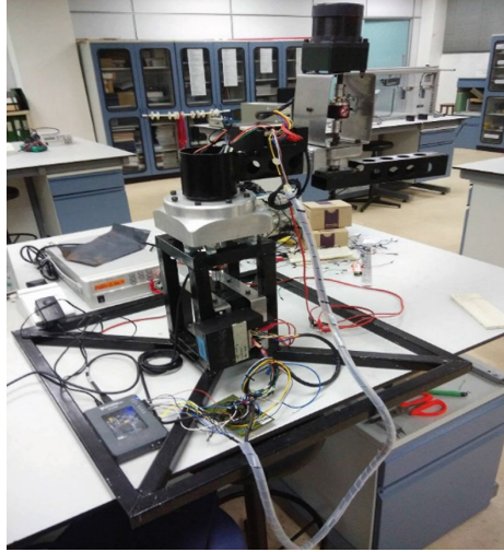
Fig. 5. The hardware of two-DOF Planar Robot Manipulator
