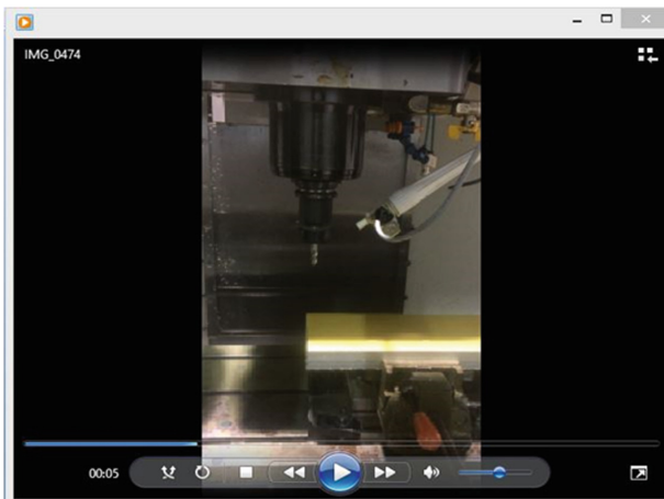
Fig. 5. Coolant stop ejecting after the designated time
