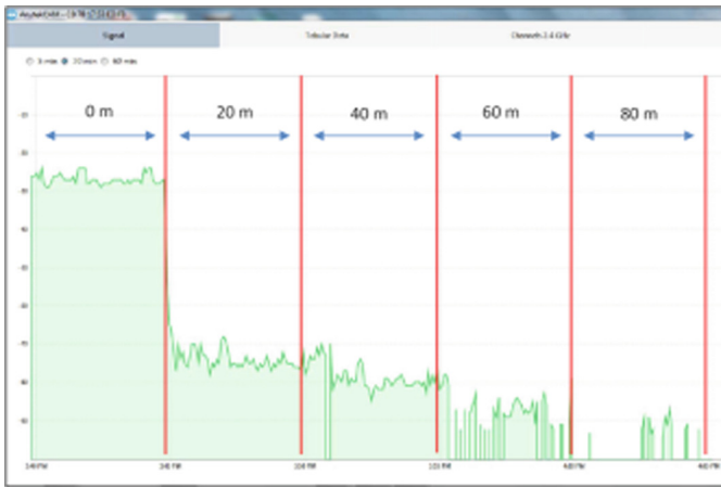
Fig. 8. Wireless camera signal coverage test
