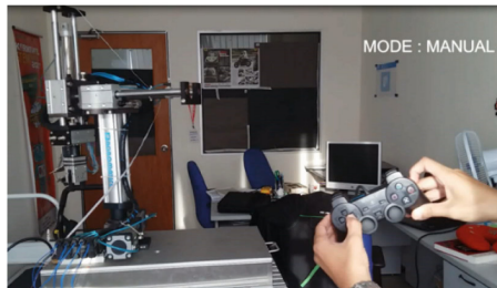
(e) The pick and place robot rotates 180° anti-clockwise by pushing button ►
