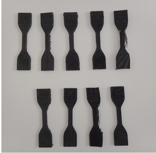
Fig. 4. Samples of dog bone ASTM D638 Type IV
