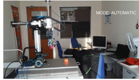
(b) The gripper grasps and lifts the red object
