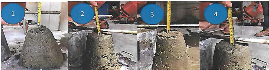
Fig. 1. Slump result (1) NC, (2) GC4%, (3) GC8% and (4) GC12%
