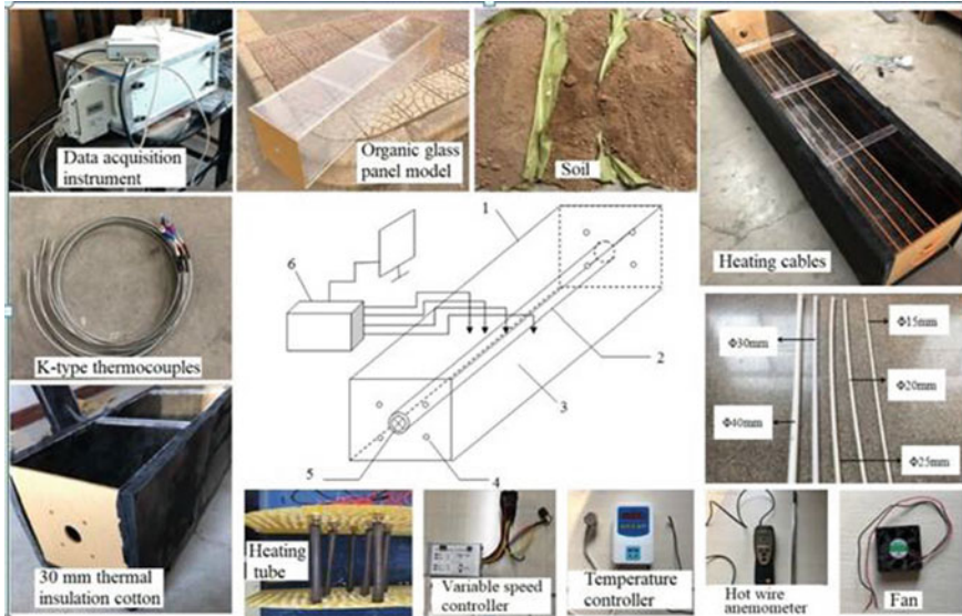
Fig. 1 EAHE model (1 Model, 2 PVC pipe, 3 Soil, 4 Mounting hole of heating cables, 5 Fan, 6 Data acquisition instrument)
