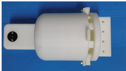
Figure 15 shows a photograph of a base link formed by assembling 3D printed base link module and female link modules. Note that a servo motor has been attached to the female part of the link. Figure 16a, b show 3D printed male and female link modules respectively.
