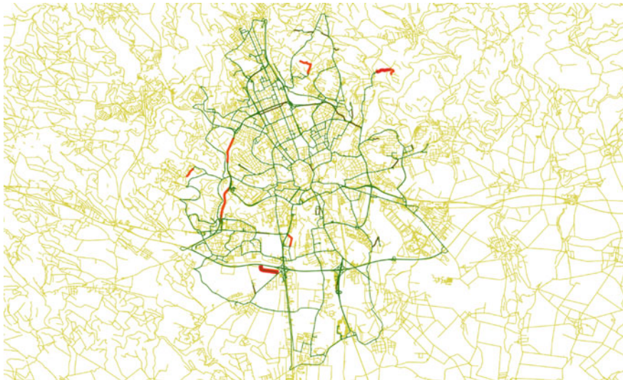
Fig. 3 Map of Brno city with traffic load from the simulator after map-matching
