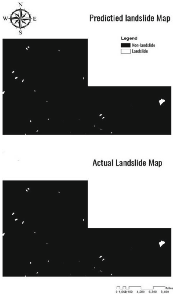
Fig. 9 Comparison between actual landslides map and the binary predicted landslides map from random forest classifier for Ratnapura study area
