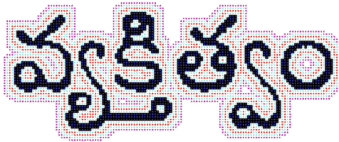
Fig. 1. Example fringe map of a word image pattern is shown. Fringe numbers are colored as 0-Blue, 1-Cyan, 2-Red, 3-Cyan, and 4-Magenta respectively. (Color figure online)
